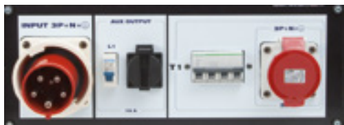
Three-phase connector (3P+N+E) of 63 A. Two additional outputs (32 A three-phase 3P+N+E and 16 A schuko mono-phase) with their own circuit breaker.
