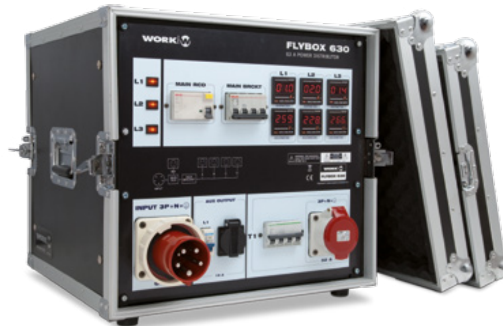
Residual current device (RCD) and general circuit breaker (4 pole). Digital voltmeter and ammeter at each phase. A light indicator shows if a phase is active.
