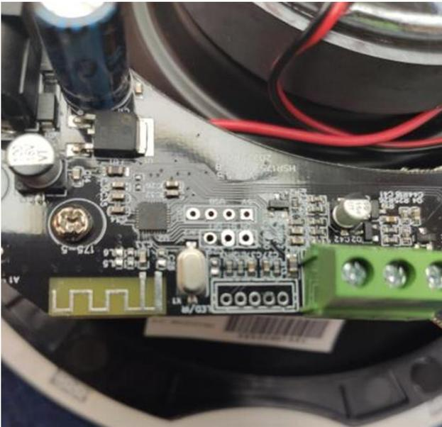
Link the holes marked BT and off by solderring them. In the picture you can see both holes marked with clamp tips.
