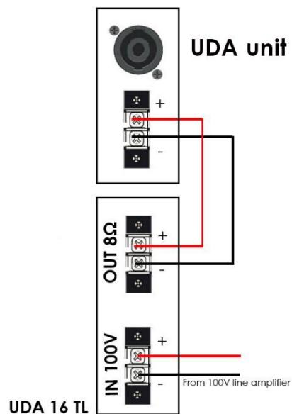
NOTE: For a better compression of the drawing, remember, UDA 8 & UDA 16 incorporate Speakon connector and barrier strip, and UDA 1, UDA 2 & UDA 4 only barrier strip
