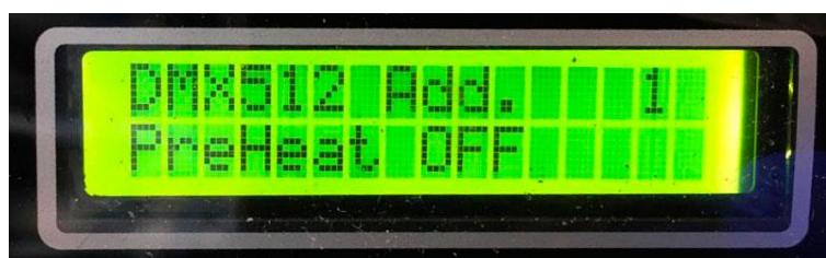
Press MENU to select the DMX mode and set the DMX start channel. Under this mode, the remote control does not work.
