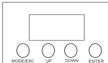
he main menu is accessed by pressing the Mode/Esc-button, Browse through the submenu by pressing Up or Down .Press the Enter-button in order to select the desired menu. You can change the selection by pressing Up or Down, Confirm every selection by pressing the Enter-button. You can leave every mode by pressing the Mode/Esc-button .The functions provided are described in the following setting.
