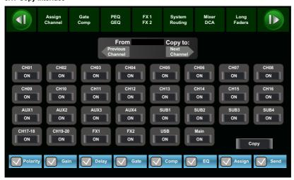
Select a channel or bus that you want to copy its settings onto other channels, then press Copy button, you can see the selected channel or bus will flash. Touch OFF of other channel or bus, it will turn to ON and the background will illuminate red,
