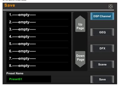
Press thisbutton to save the selected channel's and bus's DSP channel setting as DSP presetting for future use. On the screen you can touch to save preset of DSP Channel, GEQ, DFX,Scene. Pleasedo as the instruction that is shown on the LCD display.
