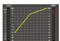
The Gate grid shows level setting of threshold in real time. Meter on the left indicates the input signal's level activity.
