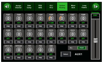
Touch it to route input channel 1 to output AUX1 as an example. Please rotate **Parameter Adjust** knob or slide long fader on the screen to change selected channel's audio level.
