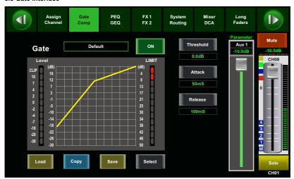
Touch the switch in this window, you can engage and disengage the Gate for the selected channel. It will illuminate to indicate that the Gate has been touched and enabled. The LCD display shows the Gate setting in real time. Its parameters can change by adjusting Threshold, Attack & Release control directly and use the **Parameter Adjust** knob to set the value.
