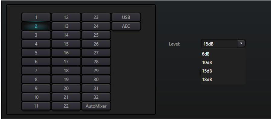
Suppression level: There are totally four levels for selection. dB here refers to the decibel of suppression noise reduction. The bigger the value, the more harm on voice generated, which is inevitable.
