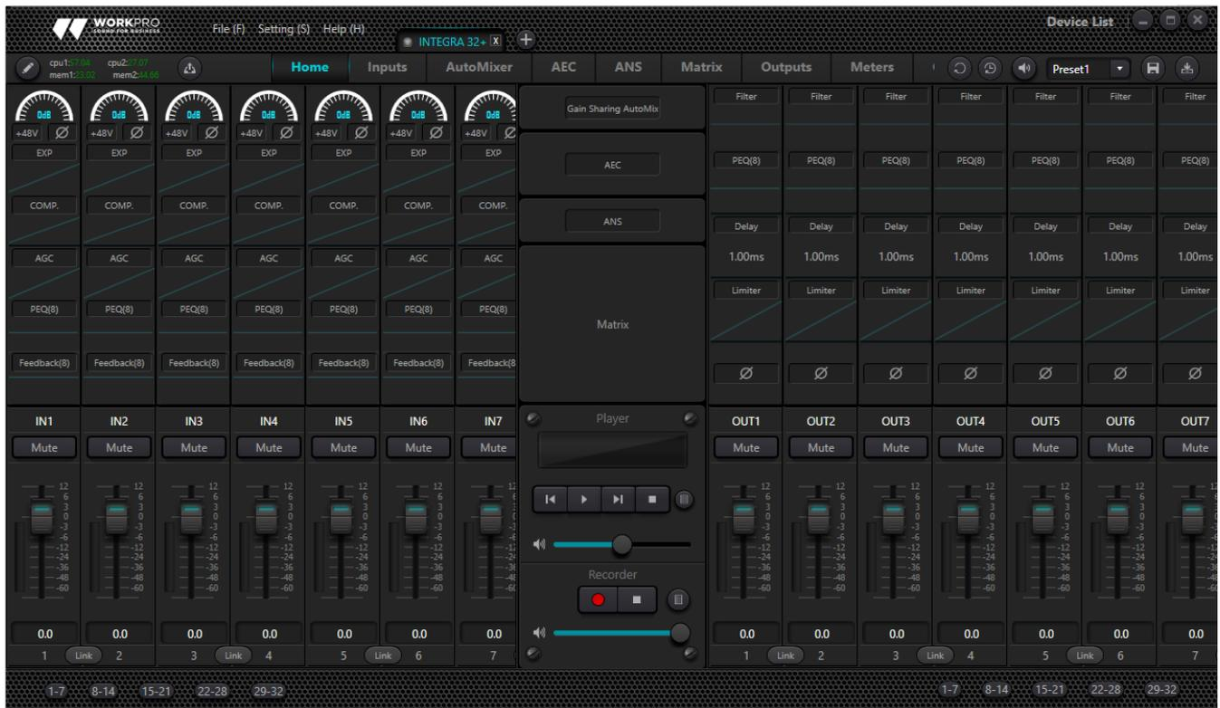
Click the button **Device List** in the right corner of the main menu and find all processors on the network automatically. The user may connect to the designated processor based on their own needs; after the connection, the indicator will flash, and one processor supports simultaneous connection and control of up to four users.
