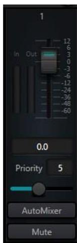
**Fader/Gain:** Sets the channel gain. Faders can be used to tell the Gain Sharing algorithm the desired relative level of each channel. NOTE: Channel gain is after the input to the AutoMix engine. Channel level may still influence the gain adjustment of other channels even if the fader is all the way down.
