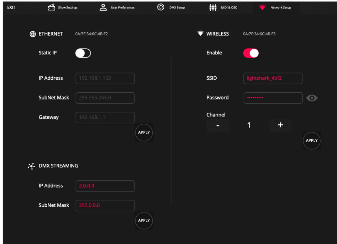
**Wireless:** Enables configuration of the integrated access point in lightShark devices. By default the network name is lightshark\_XXXX, where XXXX refers to the last 4 digits of the MAC Address of the lightShark wireless interface.
