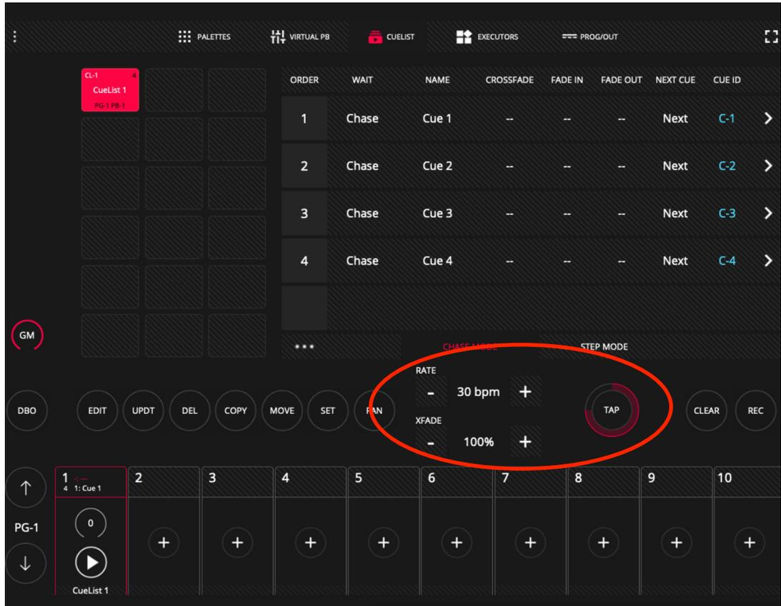
To adjust the BPM, press the TAP button repeatedly until the ring is complete.,
