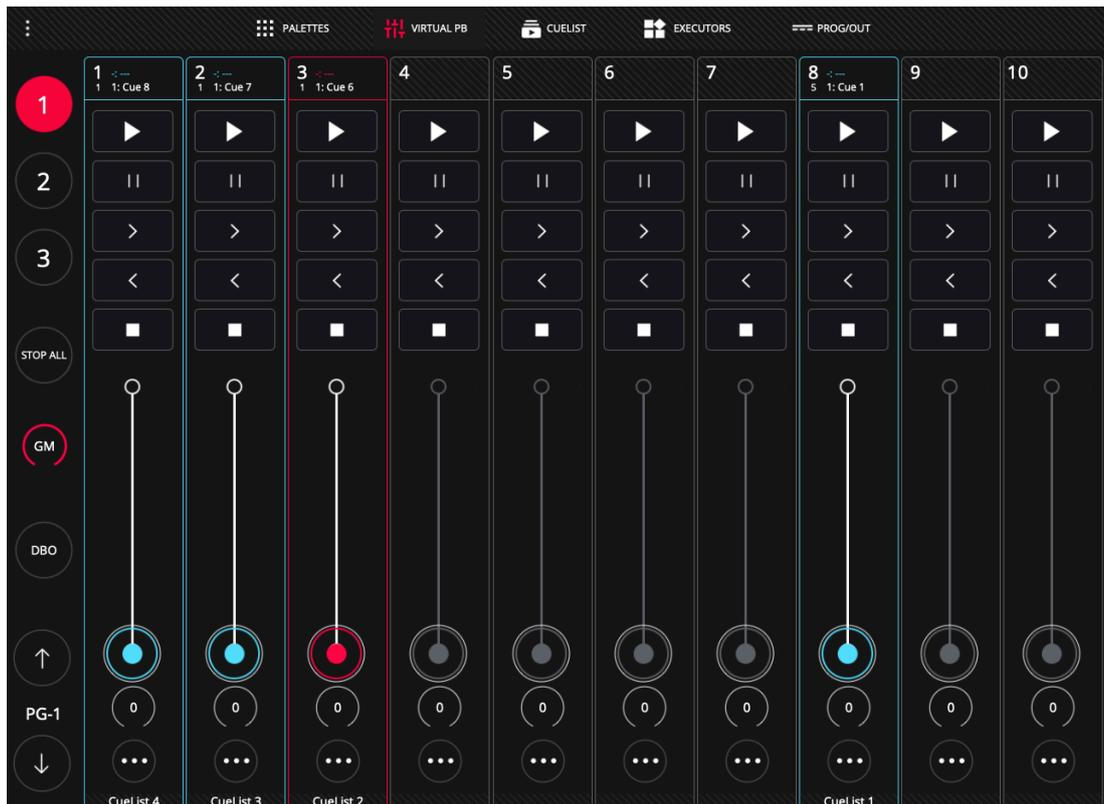
LightShark's interface is multi-touch, so you can operate multiple Playbacks simultaneously from one tablet or any device with this technology. From the buttons the user can directly access the desired Wing without scrolling.
