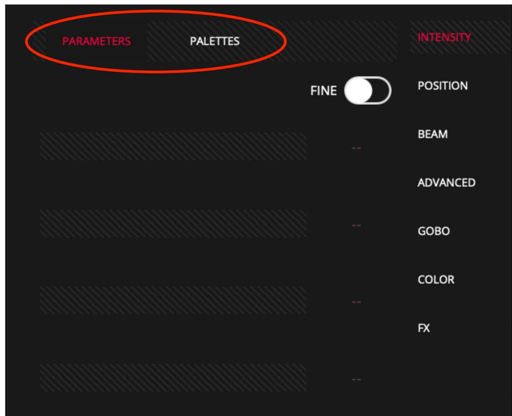
In the parameter view the user will find all parameters of the selected type. By default the parameters are always shown in blocks of 4, if the selected device has for example 7 channels of type "BEAM" it is possible to access the next 3 by scrolling vertically with your finger. Or by clicking again on the parameter button on the LS-1.
