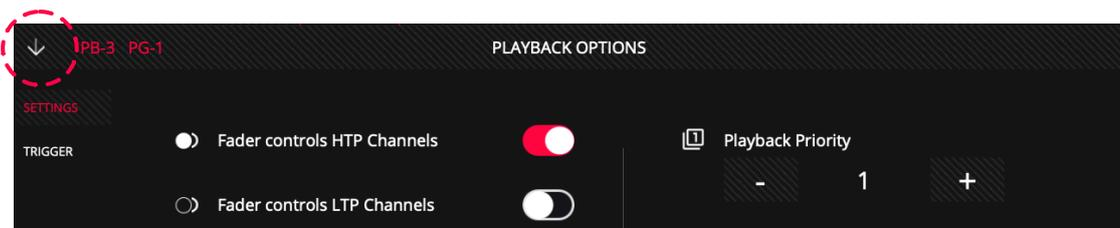
**Fader Controls HTP Channels:** When this function is activated the playback fader proportionally controls the level of all HTP channels of the current Cue from 0% to 100%. This option is activated by default.
