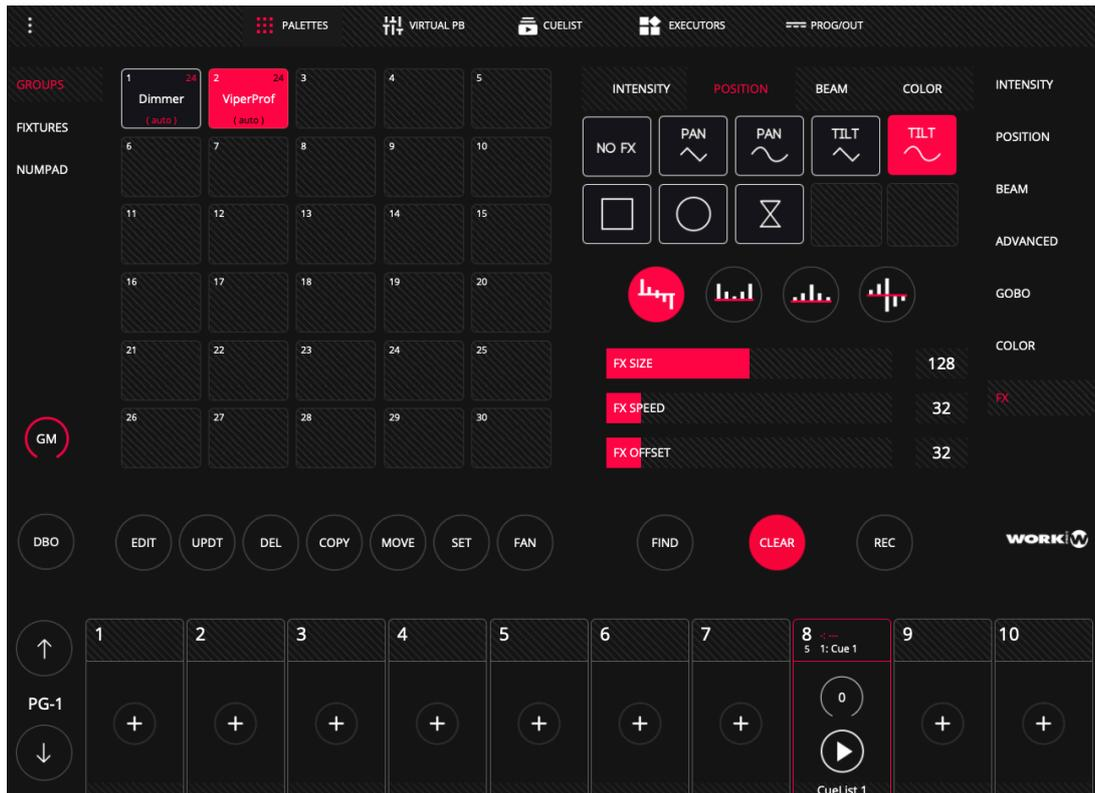
It is possible to add several effects to a fixture (or groups of fixtures) that make use of different attributes, for example, the user can add a Pan effect and also add an effect of Intensity and an effect of change-color.
