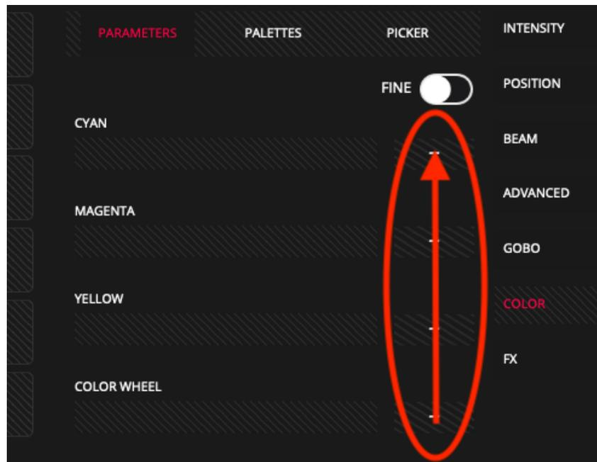
Users with an LS-1 can interact with the interface using the encoders and buttons, so that each LS-1 encoder controls each of the currently visible interface parameters (the upper parameter is controlled by the first encoder starting from the left, and so on).
