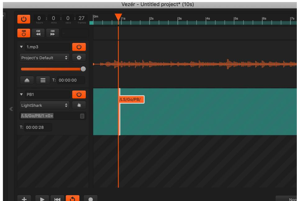
Note that actions in LightShark are performed by releasing the button, so the message is sent on <0> value instead of <1>.
