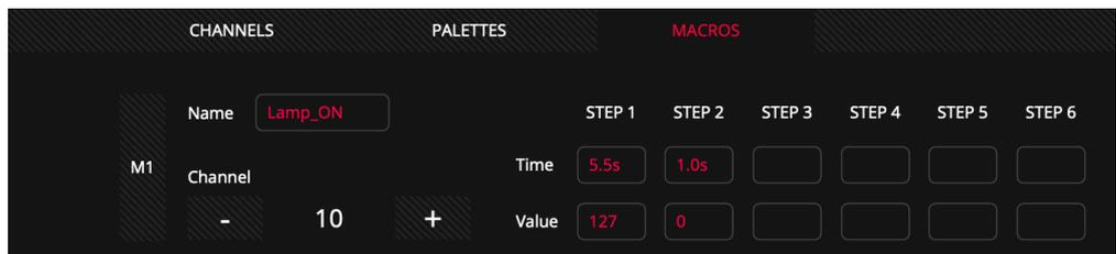
In this example the macro will send a value of 127 to the device for 5.5 seconds and then reset the channel to 0.
