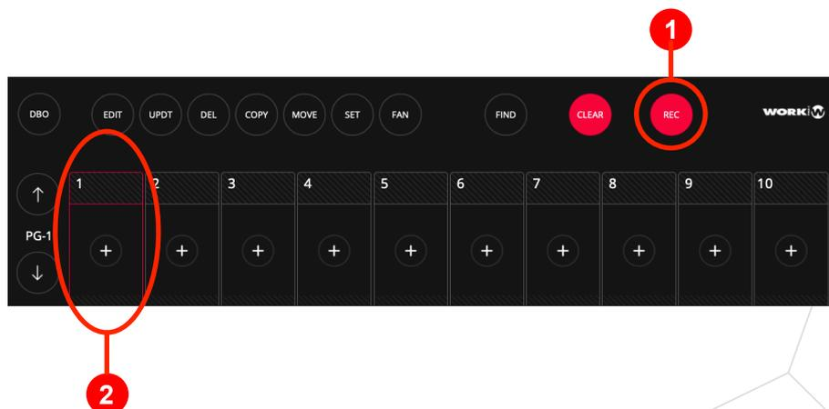
**10** Press the "CLEAR" button to clear the programmer information. You can now adjust the level through the PB-1 Fader.
