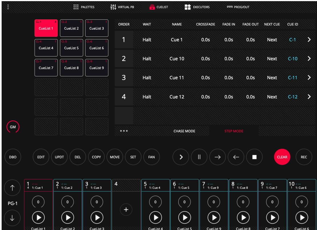
From the playbacks it is possible to directly access the cuelist on that playback via a "double click" on the top of the Playback.
