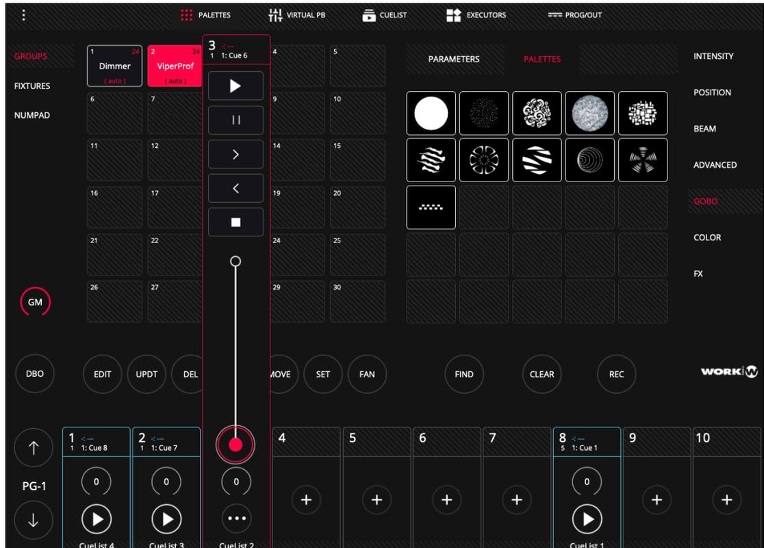
It is possible to enter a specific level into a PlayBack by holding down the value field for 2 seconds.
