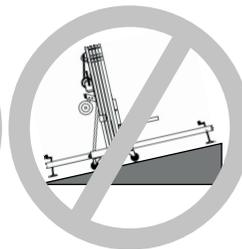
Place the tower over a flat and stable surface. Do not install it in a place where the use over the stabilize leg would not be enough to reach a perfect balance.
