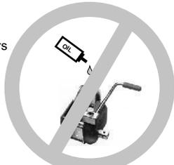
Do not lubricate the brake system of the winch, the mechanism could lose efficiency.
