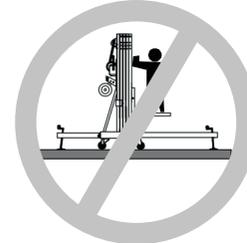
This tower is not designed to elevate persons. Do not use it for a different purpose that it has been designed
