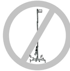
Do not move away the stabilizer legs after the load is elevated.
