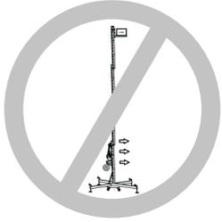
Do not move the tower after the load is elevated
