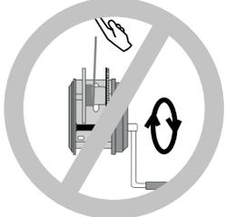
Do not catch the cable during the elevation or folding process.
