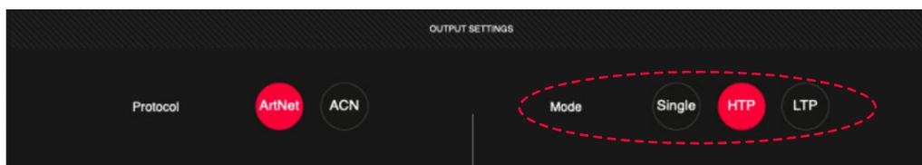
In this mode the ArtNet/ACN input of 2 universe is mixed and converted to DMX. When merging the two universes it is possible to select the type ( HTP or LTP ):
