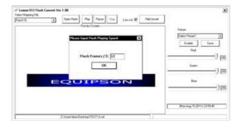
After setting the value of Frames / S click "OK" and give the name of the .Scn file that we create, once assigned the name, press "Save":
