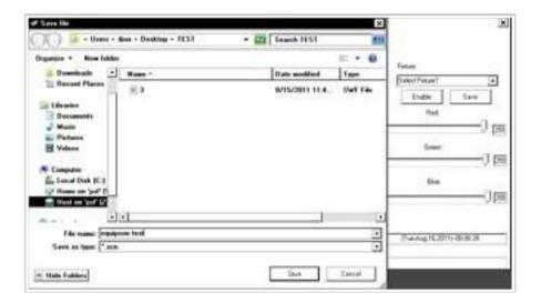
After the conversion, copy the created .Scn file to a USB memory, in the path \ \ WORK1248 \ DMXBASE. Now we can connect the USB to DMX console and update the Base from the MENU.
