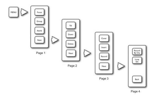
LightOn console allows the operator to lock the memory of it, allowing you to save different configurations and thus prevent unauthorized modification.
