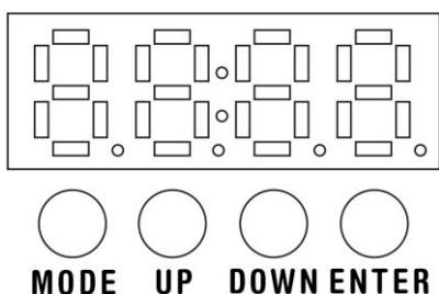
Press the MENU button (once or several times) until you get to the desired mode ( DMX, , auto or audio modes and speed control) and press enter to confirm your selection.
