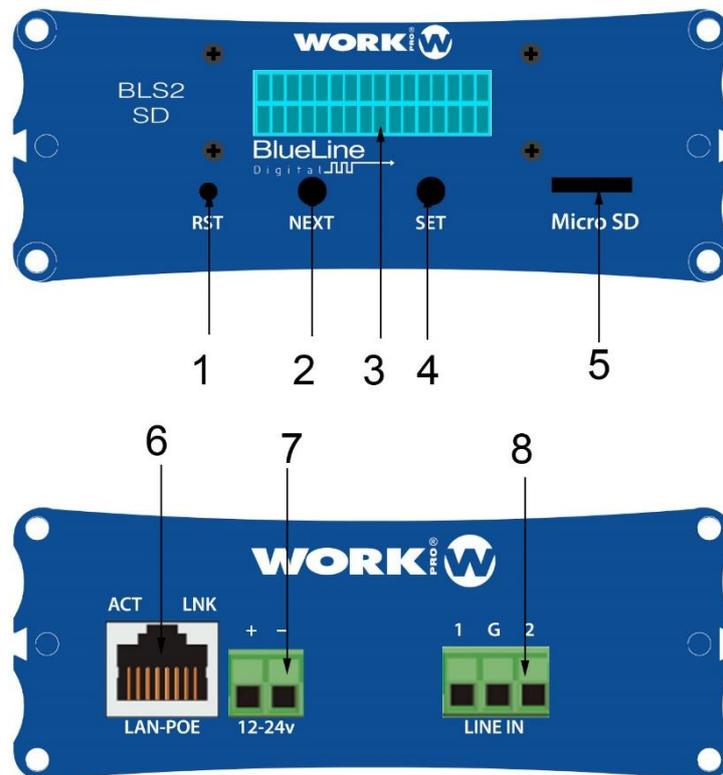
1. **Reset button.** Take the device to its factory configuration
