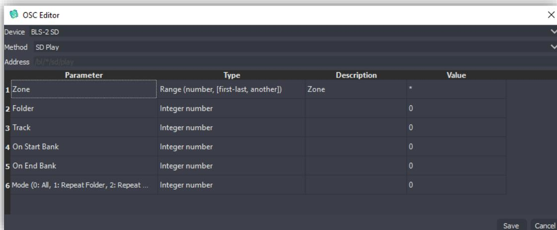
**Zone.** Normally we will select "0" in this field, it means all zones. All devices have associated a zone number, for senders it is "-1" by default. So, if we send an OSC command to a unicast IP address (BLS2 SD MKII IP address), when the command arrives to the BLS2 SD MKII, it will be processed due zone "-1" is included in all zones.
