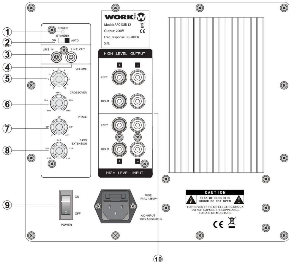
1. **Power Indicator:** Lights when the subwoofer is powered.
