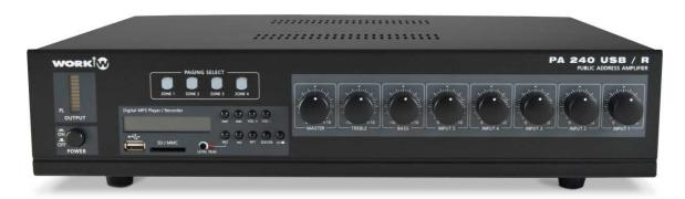
PA 240 USB/R is a 240W power amplifier that features a 5 input mixer and 4 different and selectable zones. It includes a solid state audio player/recorder(USB/SD) compatible with standard formats (MP3, WMA). It is possible to record voice messages and then play them back. The device support USB and SD storage devices with up to 32 GB memory.
