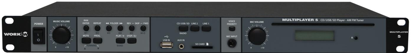
**MULTIPLAYER 5** integrates in 1 HU 19" rack, a CD player of several formats, receiver AM/FM and mixer MIC/LINE. This huge versatility give a device suitable for fixed installations or mobiles when it is not required all the elements separately to obtain the desire result. Also built-in a RS 232 connection for the reception of control commands.
