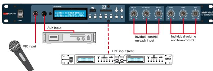
• Connection example exploiting the MIC, AUX LINE and external ports plus USB and SD.
