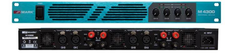
The M 4300 is a 4 channels power amplifier capable of delivering up 1600W in total. Each channel has in the rear part a XLR input and a potentiometer on the front to adjust the volume.
