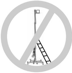
Do not lean elements (like stairs, platforms, scaffoldings, etc.) over the tower which can make pressure over it and to destabilize
