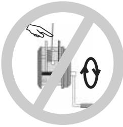
Do not catch the cable during the elevation or folding process.
