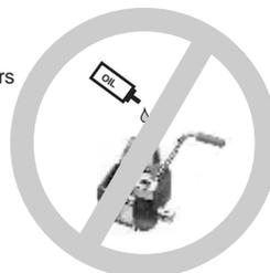
Do not lubricate the brake system of the winch, the mechanism could lose efficiency.
