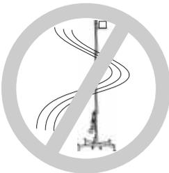
Do not use the tower in heavy wind conditions. Take into account that if the exposed height and surface is maximum, the tower stability is reduced.
