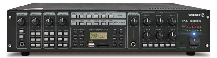
6 inputs/ 6 zone output amplifiers to create a 6x6 matrix to allow delivery of any inputs to any outputs. Each inputs has its own volume control and output selection through switches. Thus, the inputs may be added in the required output.
